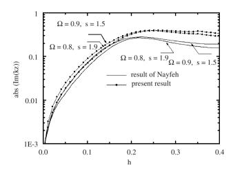
Fig. 3. Variation of the attenuation rate with liner thickness,  $\sigma = 12.92$  and  $\omega = 4$ .
