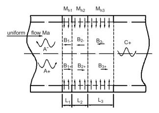
Fig. 7. The geometry of segmented non-locally reacting liners,  $L_1 = 0.15 \text{ m}$ ,  $L_2 = 0.25 \text{ m}$ ,  $L_3 = 0.40 \text{ m}$ , a = 2 mm,  $r_1 = 1.0 \text{ m}$ ,  $r_2 = 1.2 \text{ m}$ ,  $\phi = 4\%$ .
