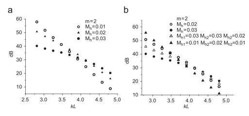
Fig. 8. Effect of the variations of frequency and bias flow on the attenuation.
