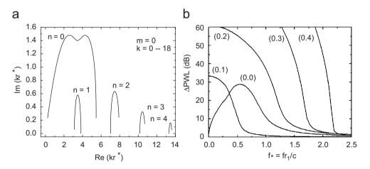
Fig. 4. Effect of frequency variation on the eigenvalues (a) and insertion loss (b),  $r_1 = 1.0$  m, h = 0.2, Ma = 0, L = 1.0, a = 3 mm,  $\phi = 5\%$ ,  $Ma(U) = U/c_0 = 0.03$ .
