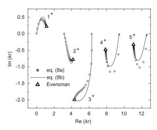
Fig. 2. The integration paths formed by using the different homotopy equations, Ma = 0.5, kb = 1.0,  $\beta_0 = 0.72 - i0.42$ .
