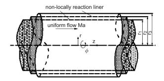
Fig. 5. A circular duct with double-layer, acoustically non-locally reacting liner circular duct.
